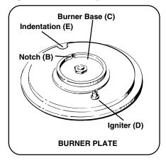
The Burner Plate has a notch (B) on the burner base, directly across from the igniter (D). This is where the tab (A) on the burner cap fits.
